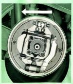
When adjusting the rear wheel brakes, the hand brake must be released. It is advisable to depress the brake pedal sharply before and after adjusting the brake shoes to ensure brake shoe centering, i.e. the proper position of the shoes relative to the brake drum.
