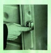
Door cylinder locks should be treated with graphite. Dip the key into the graphite, insert key and move it back and forth several times.
