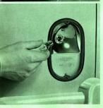
Replacing Rear Turn Indicator Bulb. Remove two Philips screws and take off lens and rubber gasket. Press bulb lightly into holder, turn and remove. Insert replacement bulb. As with the front turn indicator, be sure the gasket is properly seated, then replace lens and tighten the screws evenly.
