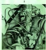
The adjustment is correct if the engine does not stall when the throttle is either suddenly opened or shut with the clutch pedal depressed. Poor idling may also be the result of damaged gaskets, loose intake manifold flanges, faulty ignition or leaky valves. Checking and adjustment of the carburetor, automatic choke and the accelerator pump should be left to an Authorized VW Dealer, who has the experience necessary for such adjustments.
