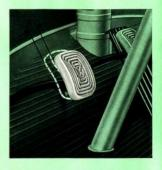
Measured at the clutch pedal this free play should be  $^{1}/_{2}^{\prime\prime}$  to  $^{3}/_{4}^{\prime\prime}$  (a). The clearance can be adjusted with the adjusting nut at the rear end of the cable.
