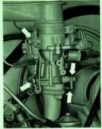
Carburetor linkage: lubricate
