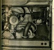
The Identification Plate is found on the vertical surface to the right of the engine.
