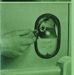
Replacing Rear Turn Indicator Bulb.
