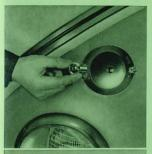
Replacing Front Turn Indicator Bulb.
