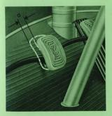
Measured at the clutch pedal this free play should be  $^{1}/_{2}^{\prime\prime}$  to  $^{3}/_{4}^{\prime\prime}$  (a). The clearance can be adjusted with the wing nut at the rear end of the cable.
