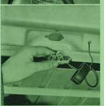
Replacing License Plate Bulb. Pull off rubber cap, press spring in holder towards bulb and remove holder. Replace bulb. Make sure that the holder contact springs are clean and that they have sufficient tension for secure bulb contact.
