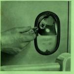
Replacing Rear Turn Indicator Bulb.
