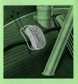
Measured at the clutch pedal this free play should be  $^{1}/_{2}^{"}$  to  $^{3}/_{4}^{"}$  (a). The clearance can be adjusted with the adjusting nut at the rear end of the cable.
