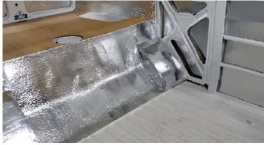
Thermal Insulation, in the whole car.
